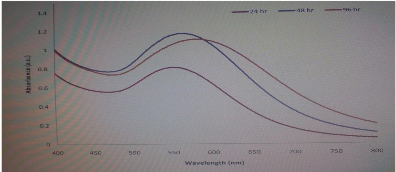
UV-Vis absorption spectra of gold nanoparticles. UV-Vis Absorption Spectra of Au NPs after Reaction of  $\text{HAuCl}_4$  with cell-free extract at pH 4 for bacterial samples
