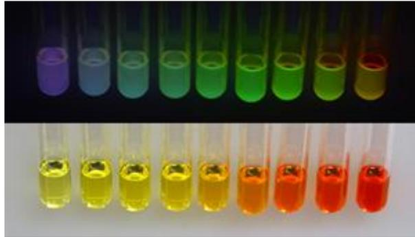
Different sized quantum dot nanoparticles are shown above, first in ultraviolet light and then in ambient light. The length of the synthesis reaction determines particle size for CdSe, increasing from left to right. In colloidal suspension, this semiconductor behaves in the same way as a metal.
