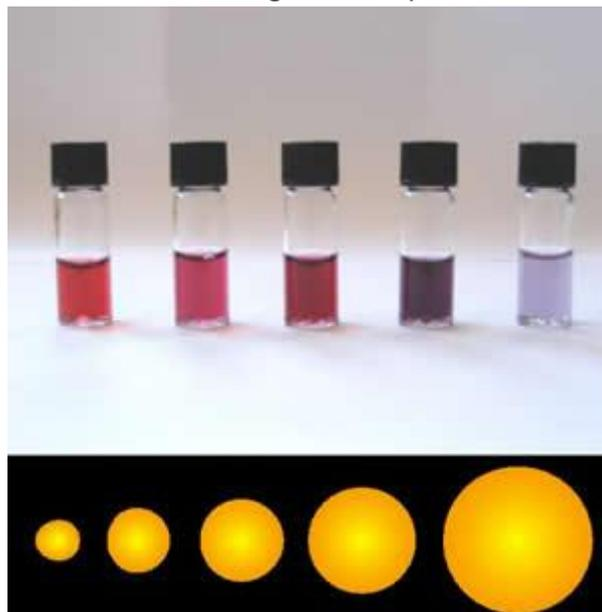
The diameter of gold nanoparticles determines the wavelengths of light absorbed. The colors in this diagram illustrate this effect.
